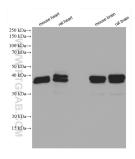
Various lysates were subjected to SDS PAGE followed by western blot with 10838-1-AP (DNAJB2 antibody) at dilution of 1:4000 incubated at room temperature for 1.5 hours.
