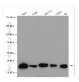
Various lysates were subjected to SDS PAGE followed by western blot with 11060-1-AP (Annexin V antibody) at dilution of 1:8000 incubated at room temperature for 1.5 hours.
