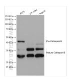
Various lysates were subjected to SDS PAGE followed by western blot with 12216-1-AP (Cathepsin B antibody) at dilution of 1:2000 incubated at room temperature for 1.5 hours.
