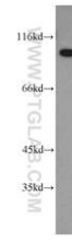
Y79 cells were subjected to SDS PAGE followed by western blot with 15975-1-AP(TELO2 antibody) at dilution of 1:1500 incubated at room temperature for 1.5 hours
