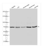
Various lysates were subjected to SDS PAGE followed by western blot with 23987-1-AP (ZBTB20 antibody) at dilution of 1:5000 incubated at room temperature for 1.5 hours.
