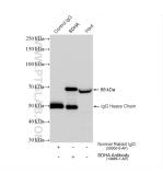
IP result of anti-SDHA (IP:14865-1-AP, 4ug; Detection:14865-1-AP 1:20000) with HEK-293 cells lysate 960 ug.
