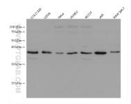
Various lysates were subjected to SDS PAGE followed by western blot with 66610-1-1g (RANKL antibody) at dilution of 1:5000 incubated at room temperature for 1.5 hours.
