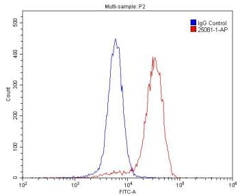
1X10<sup>6</sup> SH-SY5Y cells were stained with 0.2ug PGP antibody (25081-1-AP, red) and control antibody (blue). Alexa Fluor 488-conjugated AffiniPure Goat Anti-Rabbit IgG(H+L) with dilution 1:1500. Cells were fixed with 4% PFA and permeabilized with 0.1% Triton X-100.
