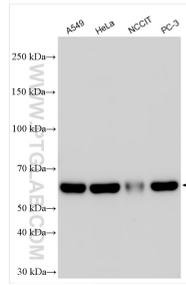
Various lysates were subjected to SDS PAGE followed by western blot with 26158-1-AP (METTL14 antibody) at dilution of 1:5000 incubated at room temperature for 1.5 hours.
