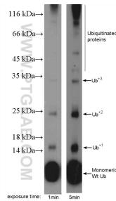
MDA-MB-453s cells were subjected to SDS PAGE followed by western blot with 10201-2-AP (ubiquitin Antibody) at dilution of 1:600 incubated at room temperature for 1.5 hours.
