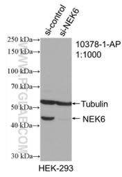
WB result of NEK6 antibody (10378-1-AP; 1:1000; incubated at room temperature for 1.5 hours) with sh-Control and sh-NEK6 transfected HEK-293 cells.
