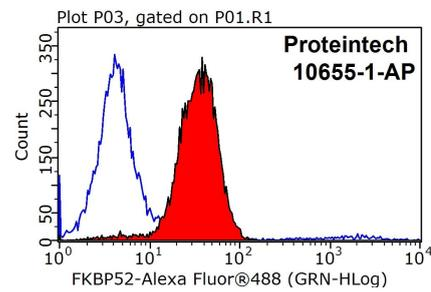
1x10<sup>6</sup> MCF-7 cells were stained with 0.2ug FKBP52 antibody (10655-1-AP, red) and control antibody (blue). Fixed with 90% MeOH blocked with 3% BSA (30 min). Alexa Fluor 488-conjugated AffiniPure Goat Anti-Rabbit IgG(H+L) with dilution 1:1000.
