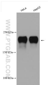
Various lysates were subjected to SDS PAGE followed by western blot with 11229-1-AP (MAP4 antibody) at dilution of 1:1500 incubated at room temperature for 1.5 hours.
