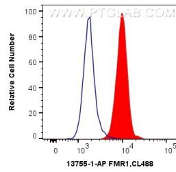
1X10<sup>6</sup> Jurkat cells were intracellularly stained with 0.4 ug Anti-Human FMR1 (13755-1-AP) and CoraLite®488-Conjugated AffiniPure Goat Anti-Rabbit IgG(H+L) at dilution 1:1000 (red), or 0.4 ug Control Antibody. Cells were fixed with 4% PFA and permeabilized with Flow Cytometry Perm Buffer (PF00011-C).
