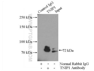
IP Result of anti-TNIP1 (IP:15104-1-AP, 4ug; Detection:15104-1-AP 1:700) with HeLa cells lysate 2000ug.
