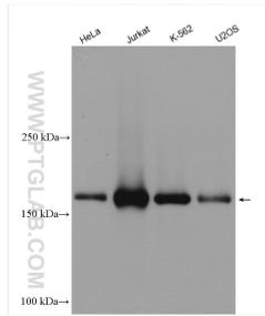
Various lysates were subjected to SDS PAGE followed by western blot with 15688-1-AP (ERCC6L antibody) at dilution of 1:3000 incubated at room temperature for 1.5 hours.
