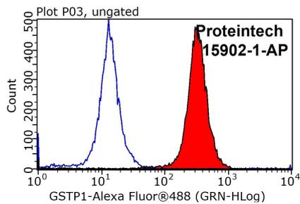
1X10<sup>6</sup> HepG2 cells were stained with 0.2ug GSTP1 antibody (15902-1-AP, red) and control antibody (blue). Fixed with 90% MeOH blocked with 3% BSA (30 min). Alexa Fluor 488-conjugated AffiniPure Goat Anti-Rabbit IgG(H+L) with dilution 1:1000.
