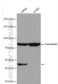
Various lysates were subjected to SDS PAGE followed by western blot with 24883-1-AP (PLEKHO1 antibody) at dilution of 1:300 incubated at room temperature for 1.5 hours.
