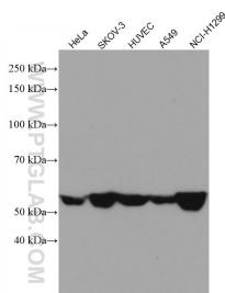
Various lysates were subjected to SDS PAGE followed by western blot with 66304-1-Ig (CD47 antibody) at dilution of 1:4000 incubated at room temperature for 1.5 hours.
