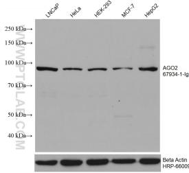
Various lysates were subjected to SDS PAGE followed by western blot with 67934-1-Ig (AGO2 antibody) at dilution of 1:4000 incubated at room temperature for 1.5 hours. The membrane was stripped and reblotted with HRP-conjugated Beta Actin Monoclonal antibody (HRP-66009) as loading control.
