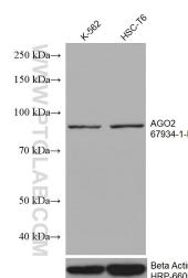
Various lysates were subjected to SDS PAGE followed by western blot with 67934-1-Ig (AGO2 antibody) at dilution of 1:4000 incubated at room temperature for 1.5 hours. The membrane was stripped and reblotted with HRP-conjugated Beta Actin Monoclonal antibody (HRP-66009) as loading control.
