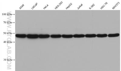
Various lysates were subjected to SDS PAGE followed by western blot with 68463-1-Ig (EIF2S2 antibody) at dilution of 1:10000 incubated at room temperature for 1.5 hours.
