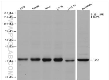
Various lysates were subjected to SDS PAGE followed by western blot with 81281-1-RR (HO-1 antibody) at dilution of 1:10000 incubated at room temperature for 1.5 hours.
