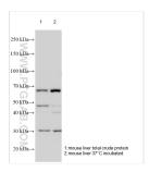
Various lysates were subjected to SDS PAGE followed by western blot with 19697-1-AP (Kv1.4-Specific antibody) at dilution of 1:600 incubated at room temperature for 1.5 hours.
