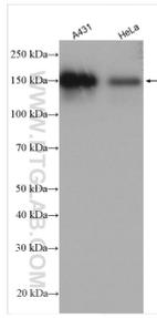
Various lysates were subjected to SDS PAGE followed by western blot with 26417-1-AP (BAG6 antibody) at dilution of 1:8000 incubated at room temperature for 1.5 hours.
