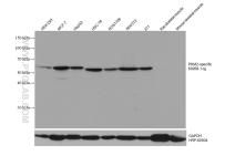
Various lysates were subjected to SDS PAGE followed by western blot with 60268-1-1g (PKM2-specific antibody) at dilution of 1:20000 incubated at room temperature for 1.5 hours. The membrane was stripped and reblotted with HRP-conjugated GAPDH Monoclonal antibody (HRP-60004) as loading control.
