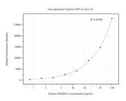
Cytometric bead array standard curve of MP50615-2, PLEKH11 Monoclonal Matched Antibody Pair, PBS Only. Capture antibody: 60453-3-PBS. Detection antibody: 60453-4-PBS. Standard:Ag13729. Range: 0.781-100 ng/mL
