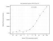
Cytometric bead array standard curve of MP51034-4, Transthyretin Monoclonal Matched Antibody Pair, PBS Only. Capture antibody: 60721-1-PBS. Detection antibody: 60721-5-PBS. Standard:Eg0931. Range: 0.098-100 ng/mL
