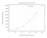
Cytometric bead array standard curve of MP51200-2, Ficolin 3 Monoclonal Matched Antibody Pair, PBS Only. Capture antibody: 60751-2-PBS. Detection antibody: 60753-1-PBS. Standard:Ag2449. Range: 6.25-200 ng/mL
