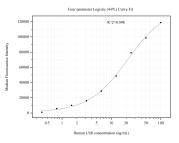
Cytometric bead array standard curve of MP51175-3, LSR Monoclonal Matched Antibody Pair, PBS Only. Capture antibody: 67508-5-PBS. Detection antibody: 67508-3-PBS. Standard:Ag13205. Range: 0.391-100 ng/mL
