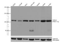
Various lysates were subjected to SDS PAGE followed by western blot with 67623-1-1g (DIS3L2 antibody) at dilution of 1:10000 incubated at room temperature for 1.5 hours. The membrane was stripped and reblotted with HRP-conjugated Lamin B1 Monoclonal antibody (HRP-66095) as loading control
