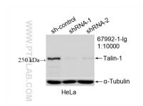
WB result of Talin-1 antibody (67992-1-lg; 1:10000; incubated at room temperature for 1.5 hours) with sh-Control and sh-Talin-1 transfected HeLa cells.
