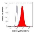
1X10^6 Jurkat cells were intracellularly stained with 0.4 ug Anti-Human LZTFL1 (68281-1-1g, Clone:2C1F6) and CoraLite®488-Conjugated AffiniPure Goat Anti-Mouse 1gG(H+L) at dilution 1:1000 (red), or 0.4 ug Mouse 1gG2a Isotype Control (C1.18.4) (65208-1-1g, Clone: C1.18.4) (blue). Cells were fixed with 4% PFA and permeabilized with Flow Cytometry Perm Buffer (PF00011-C).
