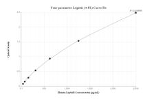
Sandwich ELISA standard curve of MP50066-1, LEPR Monoclonal Matched Antibody Pair, PBS Only. Capture antibody: 68703-1-PBS. Detection antibody: 68703-2-PBS. Standard: Ag29621. Range: 39.06-2500 pg/mL
