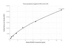
Cytometric bead array standard curve of MP01314-2, POLR2K Recombinant Matched Antibody Pair, PBS Only. Capture antibody: 82995-2-PBS. Detection antibody: 82995-1-PBS. Standard: Ag33765. Range: 0.313-20 ng/mL
