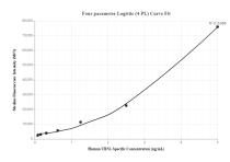
Cytometric bead array standard curve of MP00095-1, UBN1-Specific Recombinant Matched Antibody Pair, PBS Only. Capture antibody: 83001-2-PBS. Detection antibody: 83001-1-PBS. Standard: SY00809. Range: 0.078-5 ng/mL
