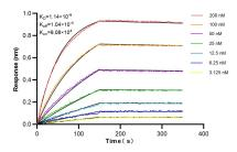
Biolayer interferometry (BLI) kinetic assays of 83495-7-RR against Human LAMR1,RPSA were performed. The affinity constant is 1.14 nM.
