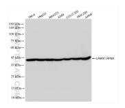
Various lysates were subjected to SDS PAGE followed by western blot with 83495-7-RR (LAMR1/RPSA antibody) at dilution of 1:10000 incubated at room temperature for 1.5 hours.
