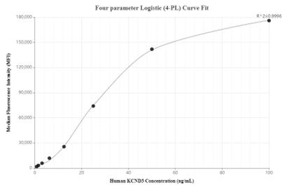
Cytometric bead array standard curve of MP00616-1, KCND3 Recombinant Matched Antibody Pair, PBS Only. Capture antibody: 83640-2-PBS. Detection antibody: 83640-4-PBS. Standard: Ag22183. Range: 0.78-100 ng/mL
