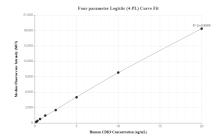
Cytometric bead array standard curve of MP00630-3, CDK9 Recombinant Matched Antibody Pair, PBS Only. Capture antibody: 83662-3-PBS. Detection antibody: 83662-4-PBS. Standard: Ag2318. Range: 0.156-20 ng/mL
