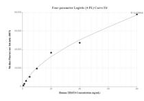
Cytometric bead array standard curve of MP00816-3, TRMT6 Recombinant Matched Antibody Pair, PBS Only. Capture antibody: 83843-1-PBS. Detection antibody: 83843-3-PBS. Standard: Ag10176. Range: 0.625-80 ng/mL
