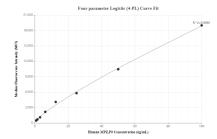
Cytometric bead array standard curve of MP00834-2, MPZ / PO Recombinant Matched Antibody Pair, PBS Only. Capture antibody: 83895-2-PBS. Detection antibody: 83895-1-PBS. Standard: Ag0848. Range: 0.781-100 ng/mL
