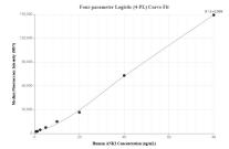
Cytometric bead array standard curve of MP00843-1, ANK2 Recombinant Matched Antibody Pair, PBS Only. Capture antibody: 83912-3-PBS. Detection antibody: 83912-1-PBS. Standard: Ag34642. Range: 0.625-80 ng/mL
