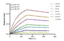
Biolayer interferometry (BLI) kinetic assays of 83947-5-RR against Mouse P-Selectin/CD62P were performed. The affinity constant is 7.97 nM.
