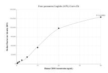
Cytometric bead array standard curve of MP00991-2, CD38 Recombinant Matched Antibody Pair, PBS Only. Capture antibody: 84070-1-PBS. Detection antibody: 84070-2-PBS. Standard: Eg0110. Range: 0.313-40 ng/mL
