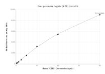
Cytometric bead array standard curve of MP00999-1, PCDH21 Recombinant Matched Antibody Pair, PBS Only. Capture antibody: 84084-1-PBS. Detection antibody: 84084-2-PBS. Standard: Ag11451. Range: 0.313-40 ng/mL
