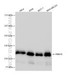
Various lysates were subjected to SDS PAGE followed by western blot with 84104-2-RR (RBM10 antibody) at dilution of 1:4000 incubated at room temperature for 1.5 hours. This data was developed using the same antibody clone with 84104-2-PBS in a different storage buffer formulation.
