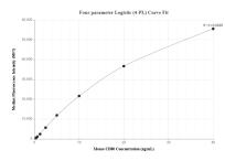
Cytometric bead array standard curve of MP01051-2, MOUSE CD80 Recombinant Matched Antibody Pair, PBS Only. Capture antibody: 84137-4-PBS. Detection antibody: 84137-1-PBS. Standard: Eg0840. Range: 0.313-40 ng/mL
