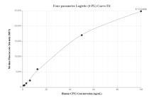
Cytometric bead array standard curve of MP01152-1, CPN1 Recombinant Matched Antibody Pair, PBS Only. Capture antibody: 84218-2-PBS. Detection antibody: 84218-1-PBS. Standard: Ag4035. Range: 0.781-100 ng/mL
