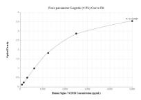
Sandwich ELISA standard curve of MP01156-2, Human Siglec-7/CD328 Recombinant Matched Antibody Pair - PBS only. 84253-2-PBS was coated to a plate as the capture antibody and incubated with serial dilutions of standard Eg1545. 84253-1-PBS was HRP conjugated as the detection antibody. Range: 78.1-5000 pg/mL
