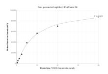
Cytometric bead array standard curve of MP01156-2, Siglec-7/CD328 Recombinant Matched Antibody Pair, PBS Only. Capture antibody: 84253-2-PBS. Detection antibody: 84253-1-PBS. Standard: Eg1545. Range: 0.313-40 ng/mL
