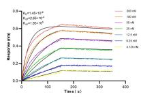
Biolayer interferometry (BLI) kinetic assays of 84335-3-RR against Human I CAM3/CD50 were performed. The affinity constant is 1.45 nM.
