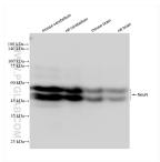
Various lysates were subjected to SDS PAGE followed by western blot with 84401-4-RR (NeuN antibody) at dilution of 1:10000 incubated at room temperature for 1.5 hours. This data was developed using the same antibody clone with 84401-4-PBS in a different storage buffer formulation.
